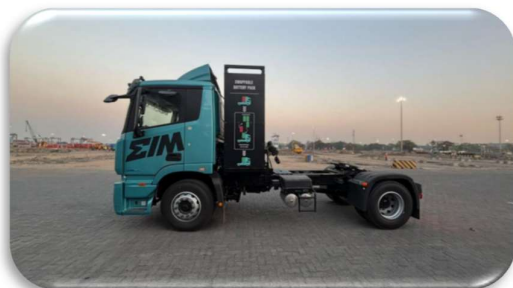
E- Tractor e-Tractor with Swappable battery pack
